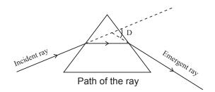
(b) A ray of white light, passing through a prism undergoes dispersion, *i.e.*, it splits into its (seven) constituent colours. These constituent colours get refracted differently. The red ray bends the least while the violet ray bends the most.
