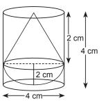
Clearly, height of the cylinder circumscribing the toy is 4 cm and its radius is 2 cm, we have Volume of the cylinder =  $\pi r^2$ H, where H is the height of the cylinder
